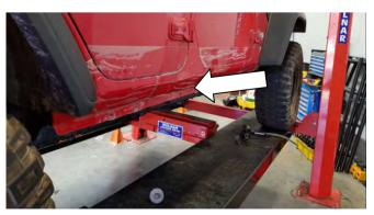
4. Protect the paint work on doors and sills both sides of vehicle. Use low tack film or similar material.
