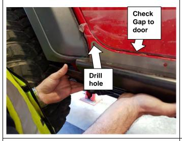
14. With the step secured against the car and the gap even use an Ø6mm drill, carefully drill hole to minimum depth at the rear of the panel as pilot for the nutsert drilling position.
