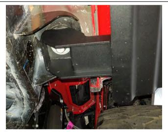
11. Fit the front mount bolt to secure the step while supporting the rear.
