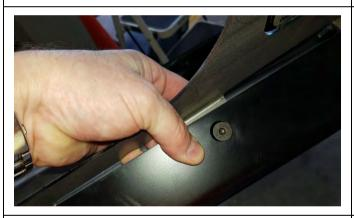
7. Fit the mount plate to the step. Start all the M8 countersunk screws
