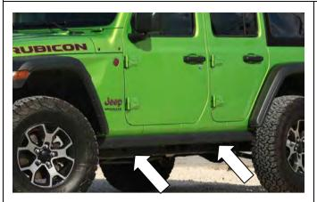
1. If fitted, remove the factory side steps retaining all fasteners.
